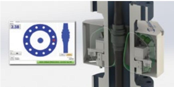
Using proprietary sensors coupled with IWS engineered software, the inVision System creates a magnetic field within the pressure containing section of the spool. The data created by the array is interpreted by the system's computers and communicated to relevant operators and machines on location.
