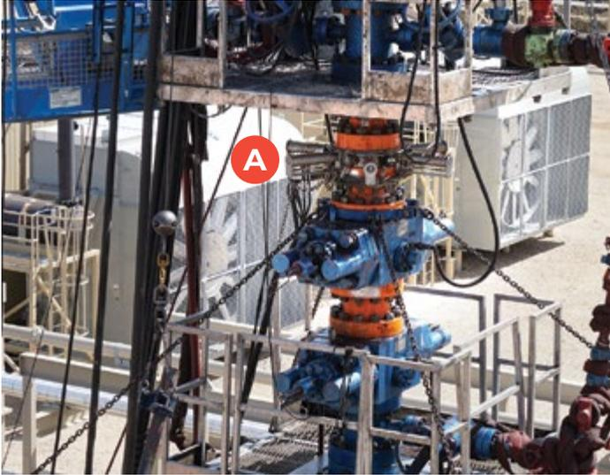
Figure 1. The inVision Spool in the stack (A)
