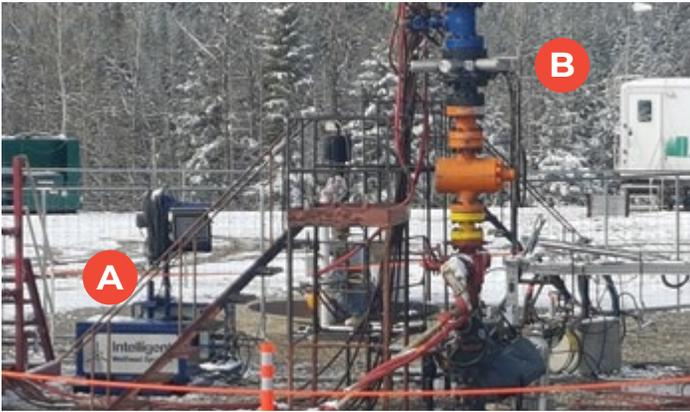
Figure 1. The inVision DAS and Skid System (A); the inVision Spool (B)
